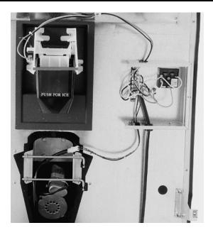
The agitation timer is located in the electrical box at the front of the dispenser.
